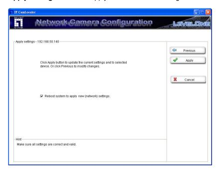
Choose "Reboot system to apply new (network) settings" to reboot after the settings are applied.
